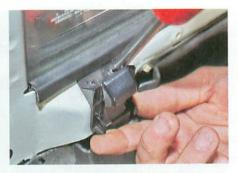
Dave noticed the door lock knob was neither upright nor central to the hole in the trim. It's easily adjusted by slackening these two screws.
