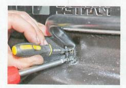
The first screw for the fixing handle was inserted after using a pick to align the other hole in the pull handle, the GRP trim and the threaded hole in the door.
