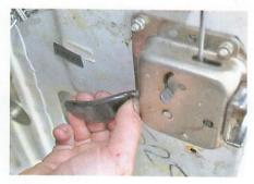
The door card is popped off its plastic trims, just as for the fronts. We bent the lever slightly, allowing it to fit through the slot in the new trim.
