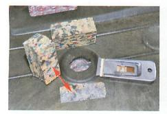
Original door casings have antivibration foam blocks on the back. To reuse them, remove with a sharp scraper (arrowed) and refit with double-sided tape.
