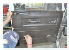
Aligning the cut-away in the trim for the door striker helped to accurately set the position at the rear. Then, the front could be raised or lowered, as required.
