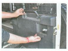
To remove this tail door card, Dave unscrewed the pull handle and clipped out the plastic plate (in right hand) allowing the latch lever enough clearance.
