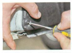
In diagonally-opposite corners, plastic rivets are removed by pushing the centre pin out. To re-use the rivets, you'll need to rescue the centre pins later.
