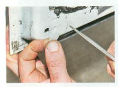
Some screw holes coincide with original fixing holes in the door. Dave filed those square with a needle file, then
