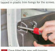
Dave fitted the new self-tapping screws to the recessed areas, one in each corner. These fixings are reinforced and the trim is more rigid than the original.
