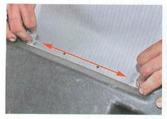
Ideal reference points of fixing holes for the door pull handle. I took a rubbing of the hole positions on the old trim, and transferred them to the new.
