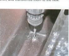
A single hole was drilled. Then the handle was temporarily fitted. The other holes were drilled using the handle as a template after checking for rubbing.
