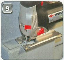
PICTURE 9 Using the Würth jigsaw to cut out the radio aperture from the front headliner section was slightly interesting. After marking out the exact size, a hole was drilled in each corner. It was only possible to saw one long cut from one side of the panel, while the other long cut had to be sawn from the other side of the panel. The short cuts had to be done by hand. It's best to protect the surface of the inside of the panel with masking tape so that the foot of the jigsaw can't damage it.
