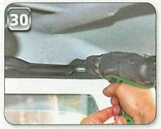
PICTURE 20 Autoglass' Russell started by fitting the main rubber section, with the joint at the bottom.
