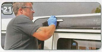
PICTURE 14 Sure enough, the aluminium strips provided some extra support so that, after the cutting out was complete, the narrow sections of GRP were not under threat. Note that, in addition to wearing the Würth facemask, I also used a vacuum cleaner to grab the dangerous dust before it got into the air.
