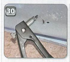
has the huge disadvantage that you won't be able to remove and refit the sun visor in future with the headliner in place. I drilled out the fixing holes and fitted rivet nuts so now, sun visor screws can be removed and refitted whenever required.
