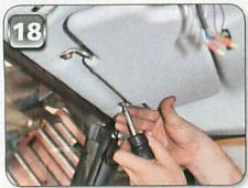
the inside of the roof. You need to make sure that the wiring can pass unimpeded. There is plenty of space between the curved corners of the headliner and those of the roof and so we made sure that any original and extra wiring was run in that area.
