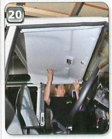
PICTURE 23 I decided that the only way of establishing where the Alpine light cut out should be made was to remove the glass from the vehicle and use the aperture to mark out the headliner.
